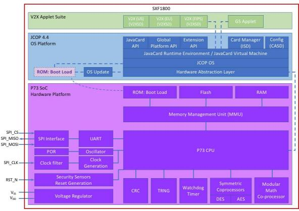
The TOE physical scope is the full integrated circuit hardware.
